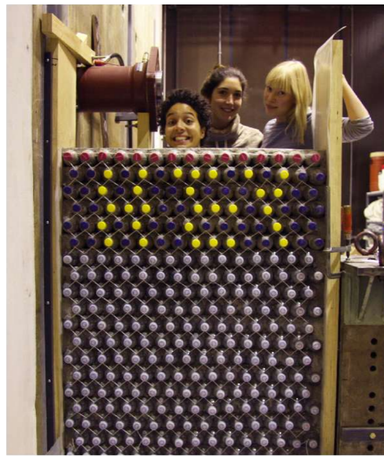
Making educational material and testing the bottle wall technique in a laboratory environment during autumn 2014.
